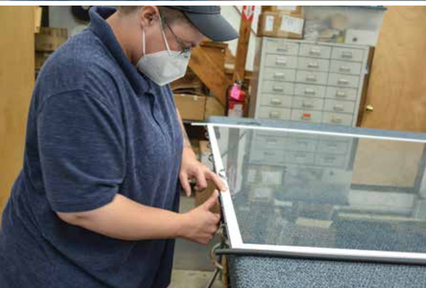
ABOVE Nearly invisible, an Innerglass window fits tightly inside the inner frame of a double-hung window, creating a sound and air buffer. Installing the windows on the inside also prevents condensation. RIGHT Kimber and David Degling have been making interior window inserts for 30 years.
