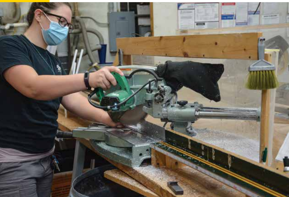
LEFT By profession a set designer, Audra Giuliano works the miter saw at the Innerglass Windows factory in Connecticut. Cutting and fitting tracks on glass windows requires precision and finesse. OPPOSITE (left, top to bottom) David Degling uses a glasscutter to score glass. When he lifts the glass up, the slight pressure causes the glass to break along the score line. • At Innerglass, Kris Earle carefully attaches springs to the edge of a window frame. • Giuliano gently taps a track in place. The tapping must be firm enough to get the glass all the way into the track; if there's too much pressure, the glass could crack.
